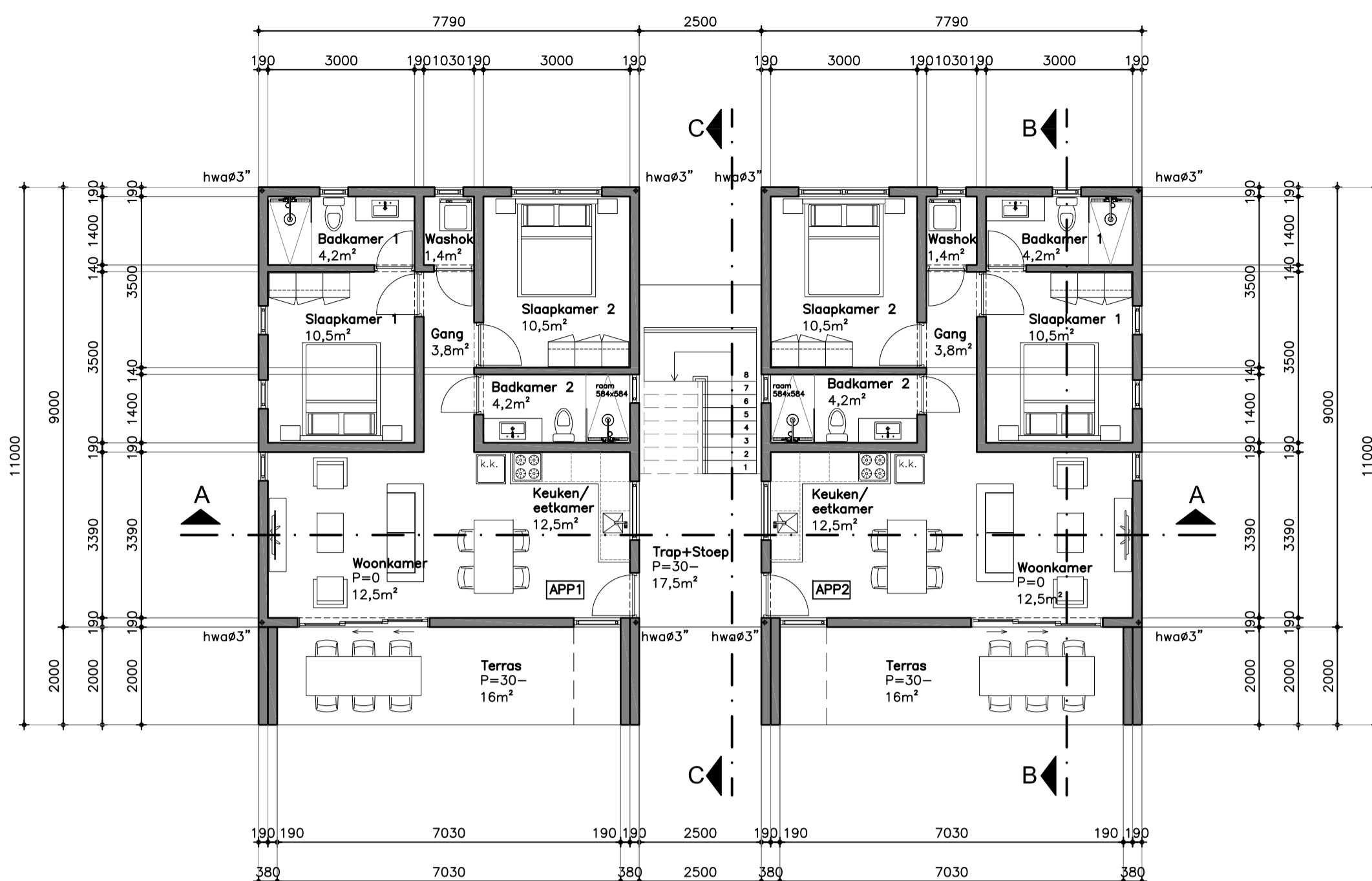
PLATTEGROND BEGANE GROND P=0 APPARTEMENT TYPE B Oppervlakte: 2 Appartementen= 2x70m 2 = 140m 2 Terrassen 2x16m 2 =32m 2 - Entree stoep+Trap =17,5m 2
